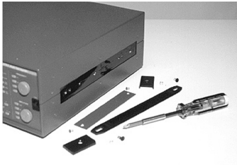
Figure B-1. Handle parts after removal
