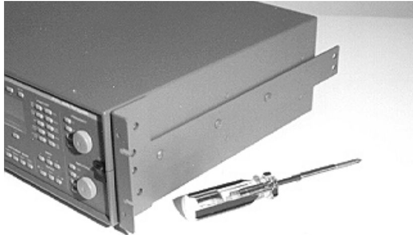
Figure B-2. Fixed rackmounting bracket in place
